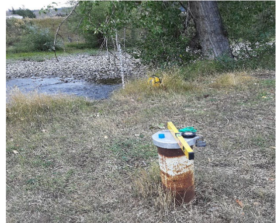
Monitoring well on the banks of Coldwater River during low water. Photo Credit: Laurie Lyons.
